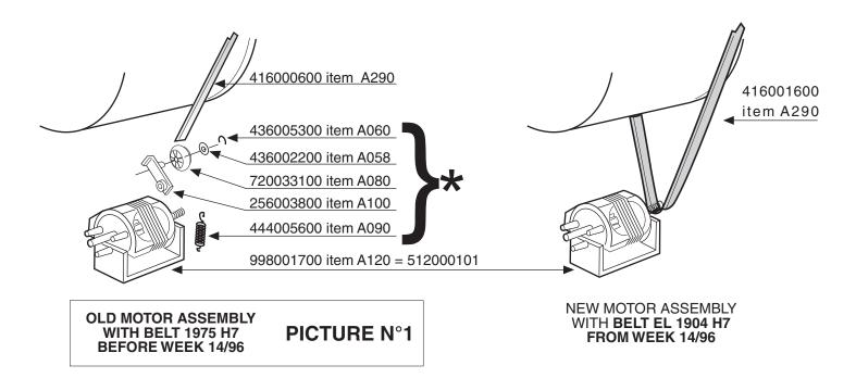
these parts together with the old belt must be removed if you use the new belt on the old products. We would like also to specify that the old items to fix the old belt will be always available like spare parts.
